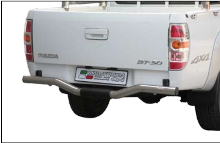
PP1/252/IX Rear Protection Ø 76 mm
